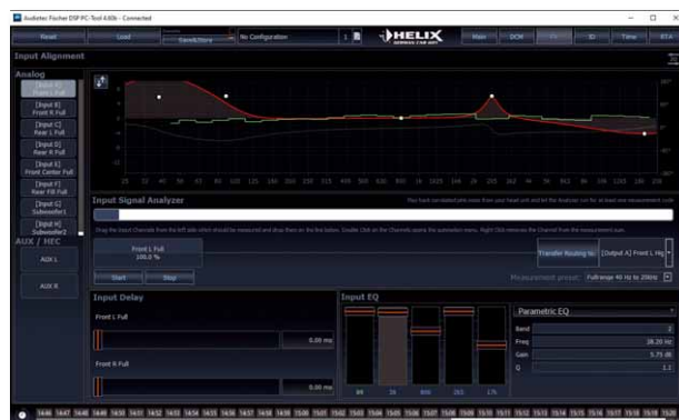
Any inputs and their sums can be measured in the ISA. EQ (with allpass) and delay correct can be measured the incoming signal
