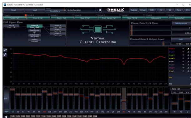
The setup of the virtual channels is the same as for the output channels, only without the crossovers. The virtual front EQ and FX front processing then affect all output channels that were routed from there
